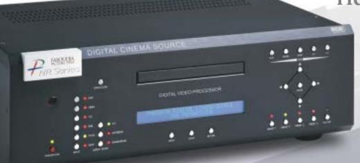
The new NRS-DCS processor maximizes the benefits of digital video and audio from DVDs by incorporating a DVD drive within a full featured Faroudja video processor. The digital video is sent directly to the internal patented digital processing stages where the signal is deinterlaced, optimized and scaled up to the display's native resolution without leaving the digital domain. Additional circuits improve edge detail and color fidelity.
