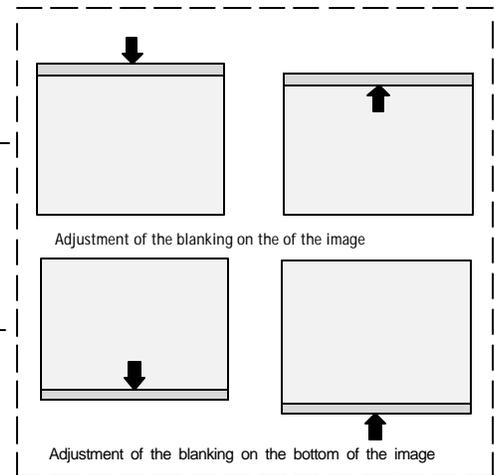
Correct by pushing the control disk forward or backward
