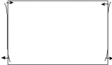
All adjustments are indicated on the screen with the function name, a bar scale and a number between 0 and 100. Adjust the next alignments until the vertical lines on the left side are straight.
