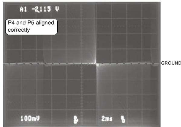
**P5: Clamping level Hor Parabola**
