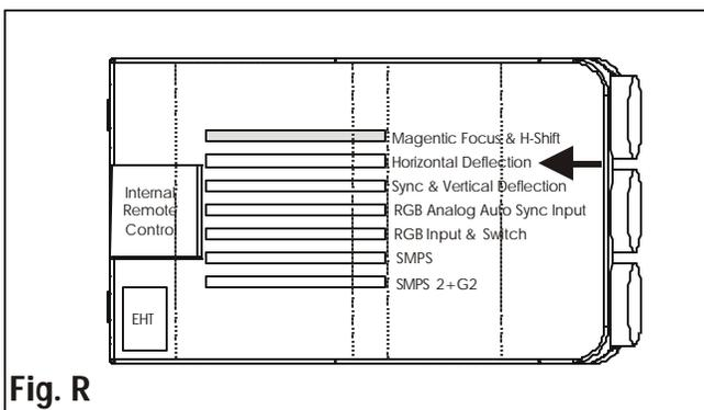
**Note:** the mentioned adjustments are Horizontal shift 'course' adjustments for the Red and Blue picture tube.
