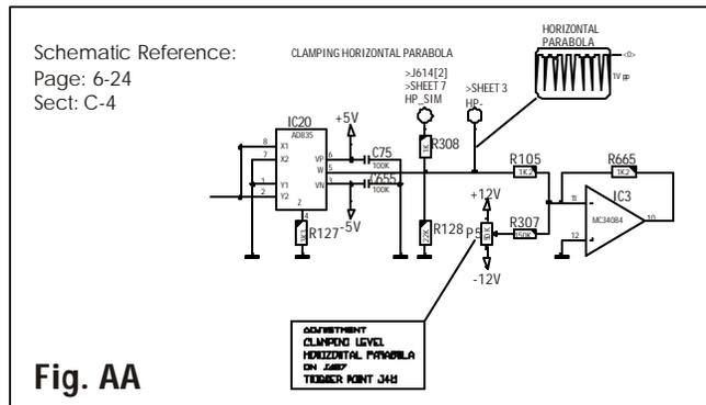
**Note:** After Adjustment of P4 and P5, readjustment of P3 is necessary.
