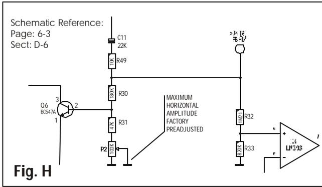
2. Connect a voltmeter to the collector of transistor Q13 on the Hor. Defl. board. Adjust potentiometer P2 for +48V on collector.
