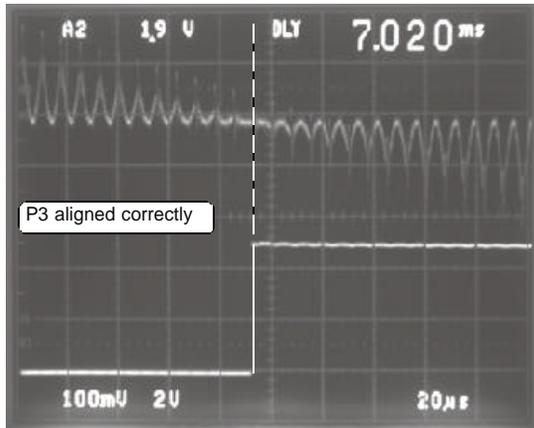
10. Connect the probe of the oscilloscope to the pin 1 of the IC30.
