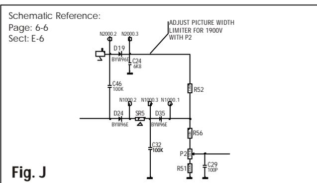
4. With respect to chassis ground, measure the dc voltage at the cathode of D19 (use a digital multimeter capable of measuring the voltage of more than 1000V). Adjust P2 **on the SM Power Supply** for 1950Vdc.
