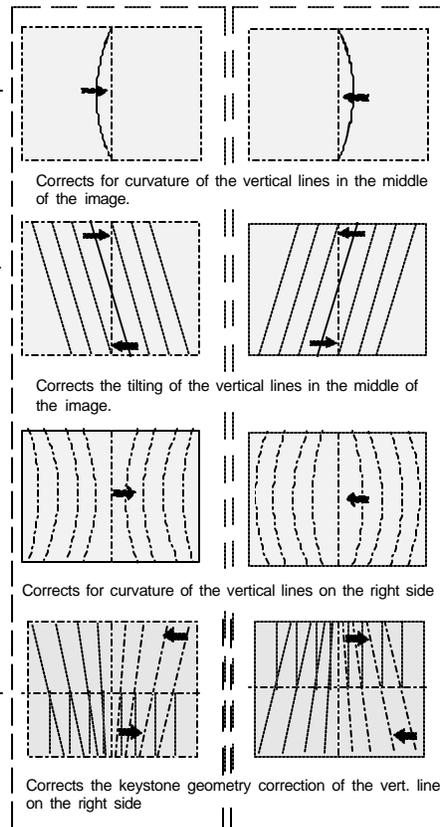
Correct by pushing the control stick to the right
