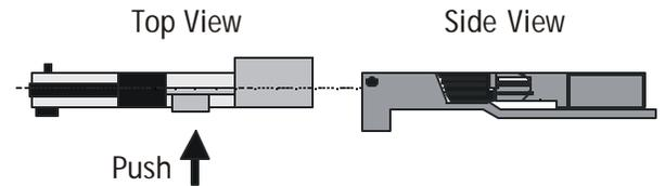
Press the board lock and lift up the module handle.
