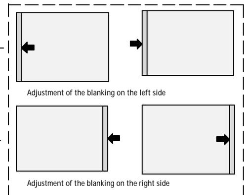
Correct by pushing the control disk to the right or to the left
