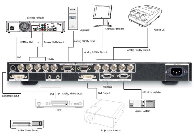
**NOTE#1:** In installations where there are multiple sources using the same connection on the DVP1080, an external switcher should be used.
