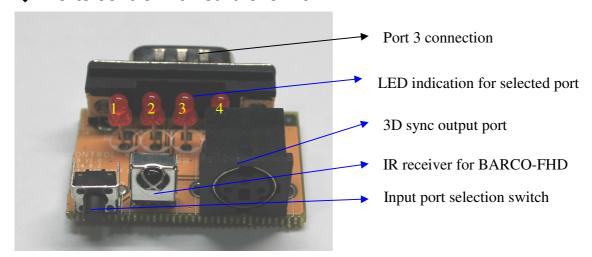
Connect control kit to Port3 to control BARCO-HD card
